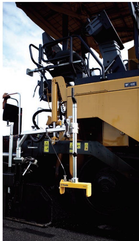
Multiple sensor readings helped ensure a smooth mat.
