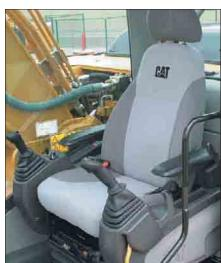
**Consoles.** Redesigned consoles feature a simple, functional design to reduce operator fatigue, ease of switch operation and excellent visibility. Both consoles have attached armrests with height adjustments.
