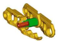
**Tracks.** The 323D comes standard with grease lubricated tracks. The track links are assembled and sealed with grease to decrease internal bushing wear, reduce travel noise and extend service life lowering operating costs. **Structures.** Proven structural manufacturing techniques, assure outstanding durability and service life from these important components.
