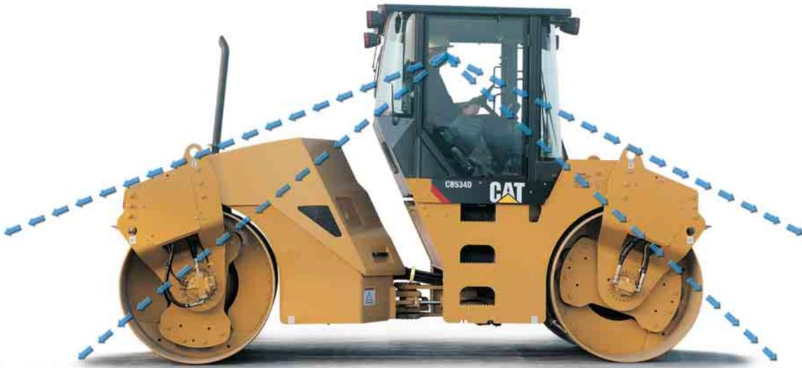
**Visibility to objects.** The visibility to objects 1 m high and 1 m in front of the machine or behind the machine.
