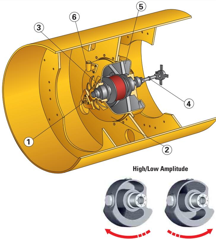
**Amplitude selections.** High or low amplitude is selected from the operator station. Direction of weight shaft determines the amplitude level.
