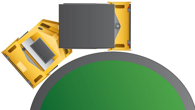
**Centered articulation.** The centered articulation with 50% of the machine length behind the pivot and 50% forward delivers evenly balanced weight front to rear. Drums track in the same path even in turns.
