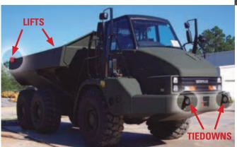
**Lift and Tiedowns** are featured on the body and front (left photo), as well as the rear (bottom photo), for secure transportability.
