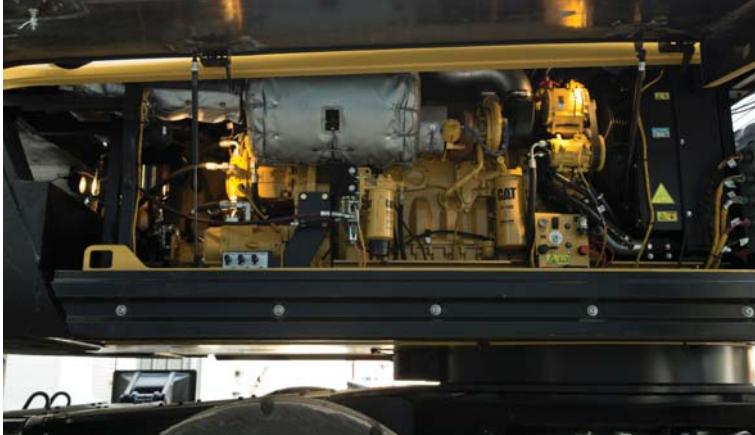
To ease serviceability on the MH3059, all primary service points are conveniently located under a single access service panel on the right side of the machine or beneath the top engine access panel. Easily locate components with the engine and cooling system's longitudinal layout. Both panels are hinged with gas struts, ensuring that one technician can easily access all maintenance points.
