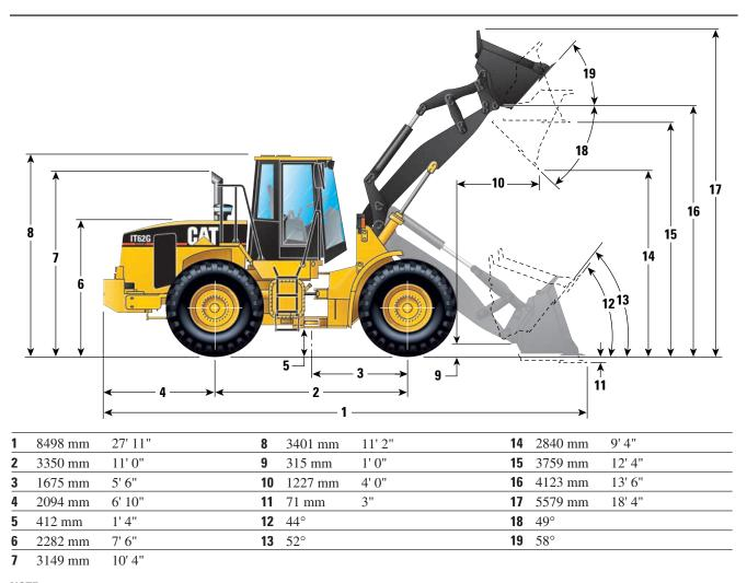
**NOTE:** Dimensions listed are for machines equipped with 23.5-R25 XHA (L-3) tires, 4.25 yd<sup>3</sup> MH bucket. \*See Operating Specifications on page 19.
